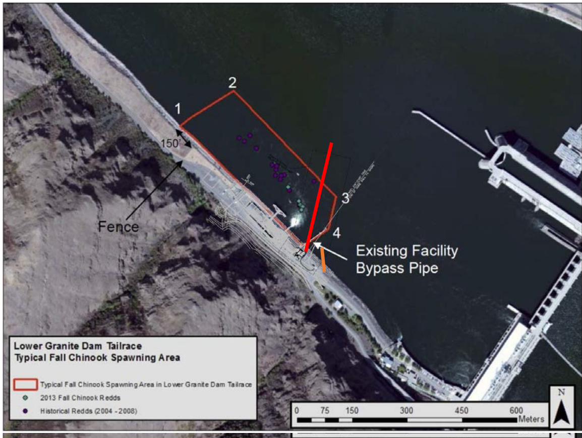
Figure 3. Typical fall Chinook spawning area in the Lower Granite Dam tailrace and new outfall construction area. The bright red line represents the new primary bypass outfall. The orange line represents the new emergency bypass outfall.
